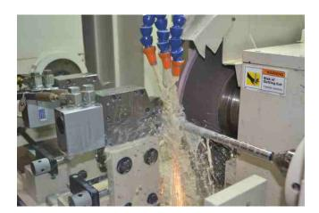
Precise Mandrel Grinding Using Cylindrical Grinding Machine (50 m/s) with CNC control and Steady Rests
